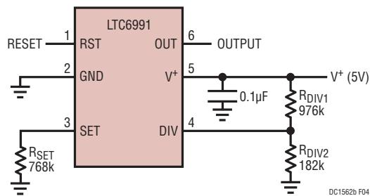
**Figure 4. DC1562B-B, 1Hz (1Sec Period) Fixed Frequency Oscillator**
