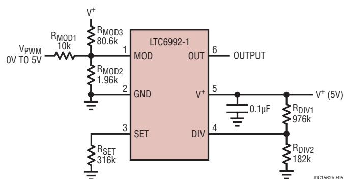
**Figure 5. DC1562B-C, 10kHz 0% to 100% Duty Cycle PWM**
