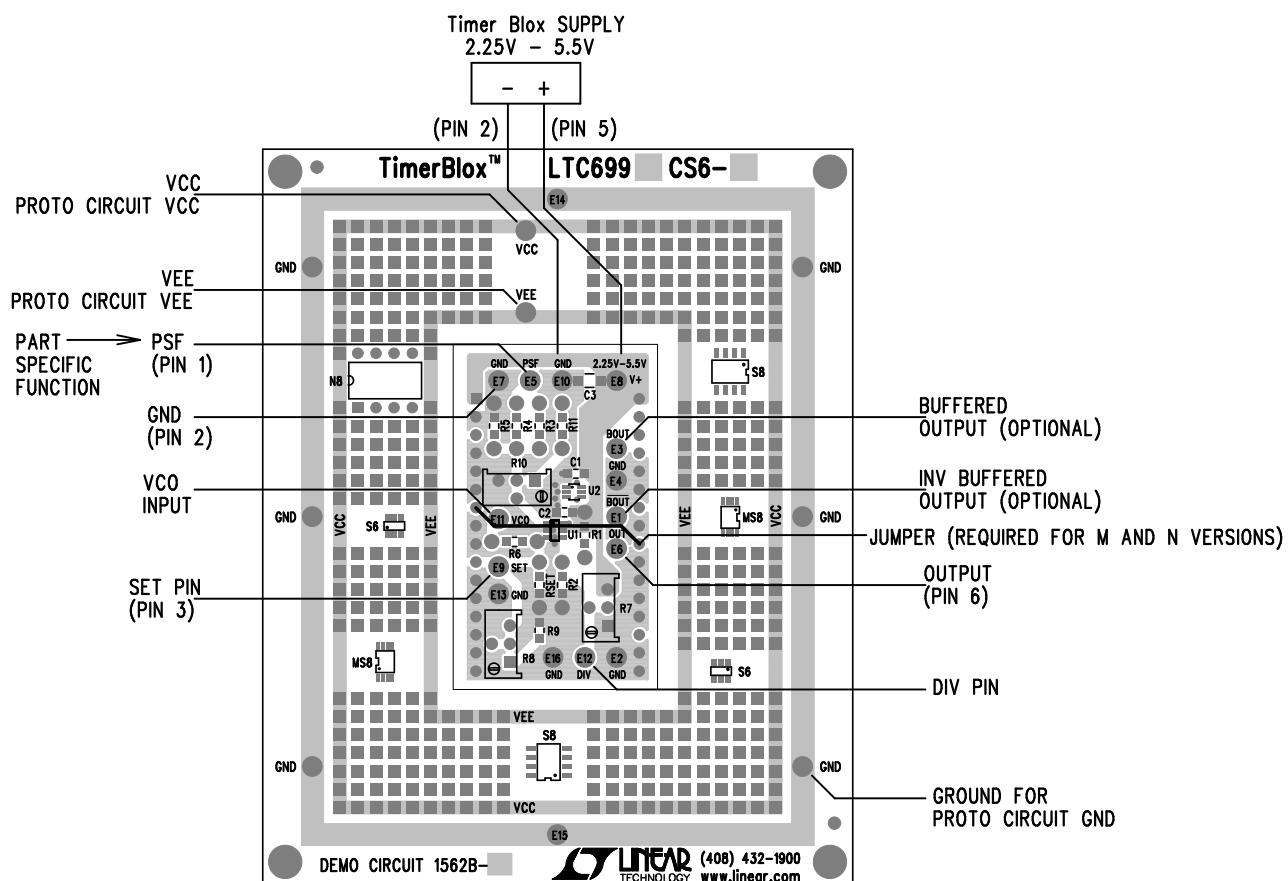
Figure 1. DC1562B-X External Connection Diagram
