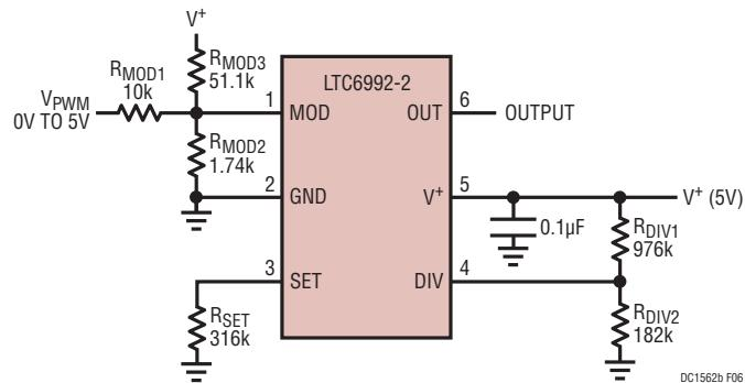
Figure 6. DC1562B-D, 10kHz 5% to 95% Duty Cycle PWM
