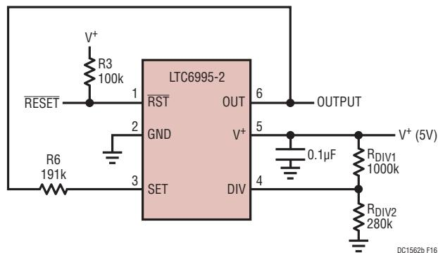
Figure 16. DC1562B-N, 1sec Active Low Power on Reset
