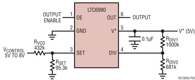
**Figure 3. DC1562B-A, 1kHz to 10kHz VCO**
