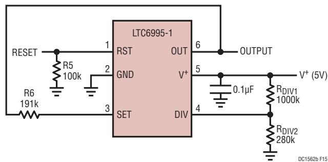
Figure 15. DC1562B-M, 1sec Active Low Power on Reset
