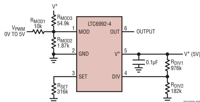
Figure 8. DC1562B-F, 10kHz 5% to 100% Duty Cycle PWM
