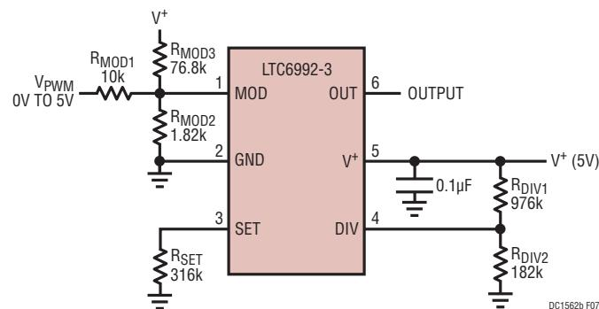
Figure 7. DC1562B-E, 10kHz 0% to 95% Duty Cycle PWM
