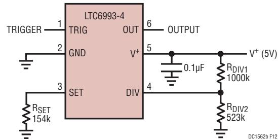
Figure 12. DC1562B-J, Falling Edge Retriggerable 100ms Positive Output Pulse One-Shot
