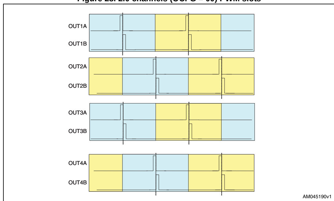
Figure 28. 2.0 channels (OCFG = 00) PWM slots
