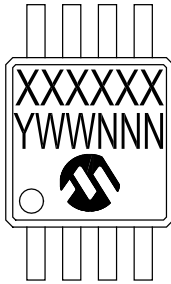
8-Lead SOIC (150 mil) (MCP661, MCP662, MCP663)
