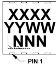
8-Lead DFN (3x3)(MCP662)
