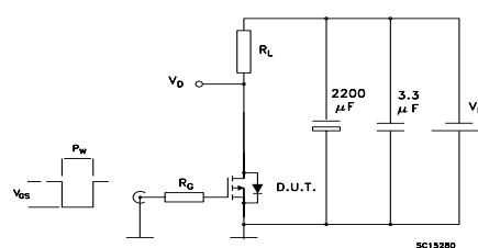
**Figure 14: Gate charge test circuit**
