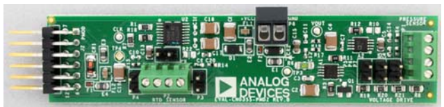
Figure 9. Photo of EVAL-CN0355-PMDZ Board
