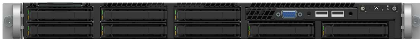
Figure 11. 2.5" Drive Bay – 8 Drive Configuration (Model R1208WFxxx)
