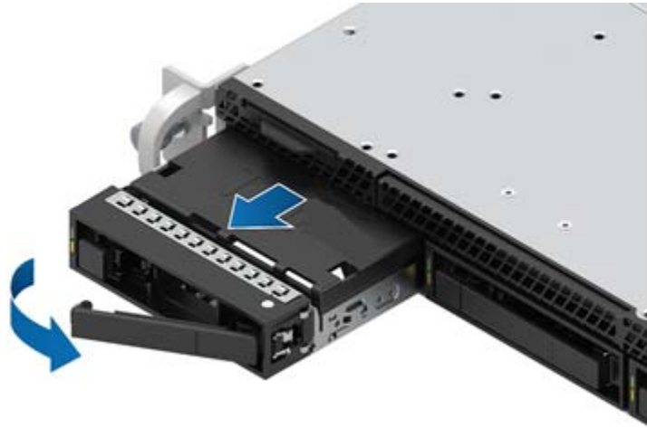
Figure 29. Drive Carrier Removal
