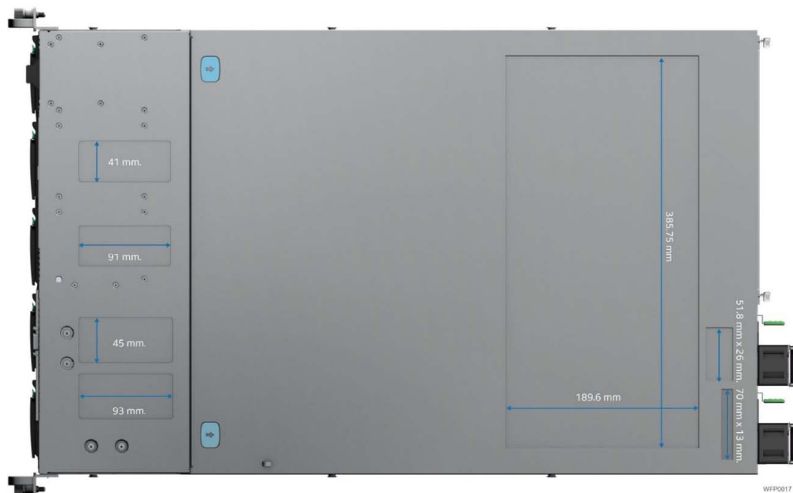
Figure 14. Label Emboss Dimensions
