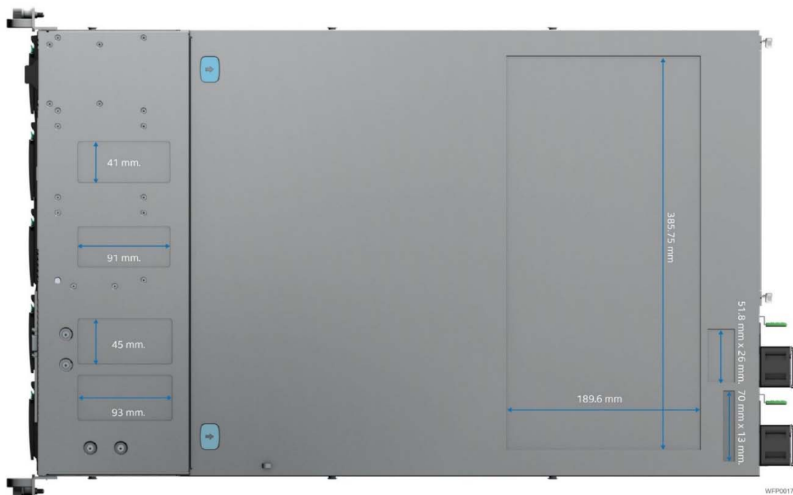
Figure 14. Label Emboss Dimensions
