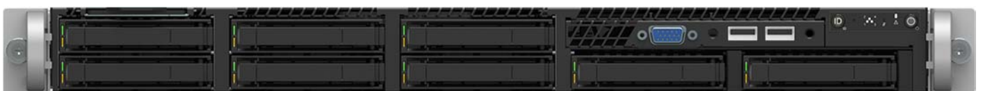
Figure 11. 2.5" Drive Bay – 8 Drive Configuration (Model R1208WFxxx)
