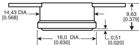
SERIES NAME 2450R Phenolic Automatic Reset Thermostat
