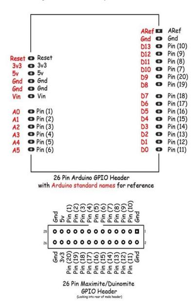
MM-BASIC allows the GPIO ports to be accessed with the PIN() command and function, and different functions to be set with SETPIN command.
