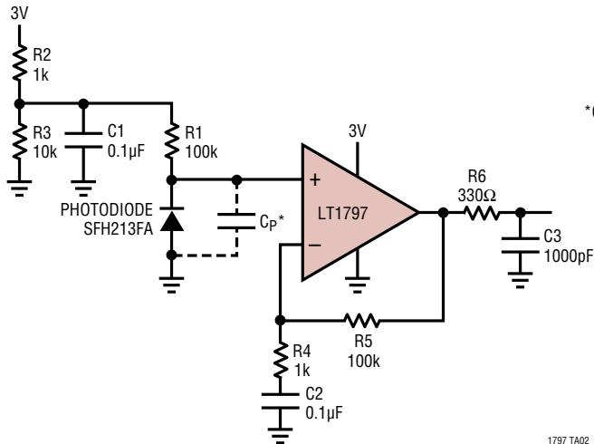
\* $C_P$  = SUM OF PHOTODIODE CAPACITANCE, PARASITIC LAYOUT CAPACITANCE AND LT1797 INPUT CAPACITANCE  $\approx 10\text{pF}$ .
