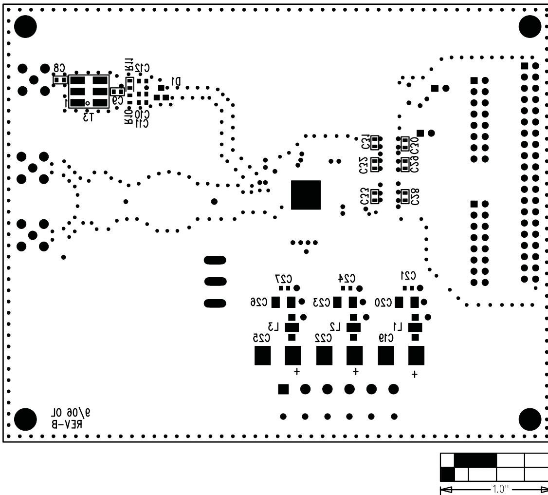
Figure 10. MAX19586/MAX19588 EV Kits Component Placement Guide—Solder Side
