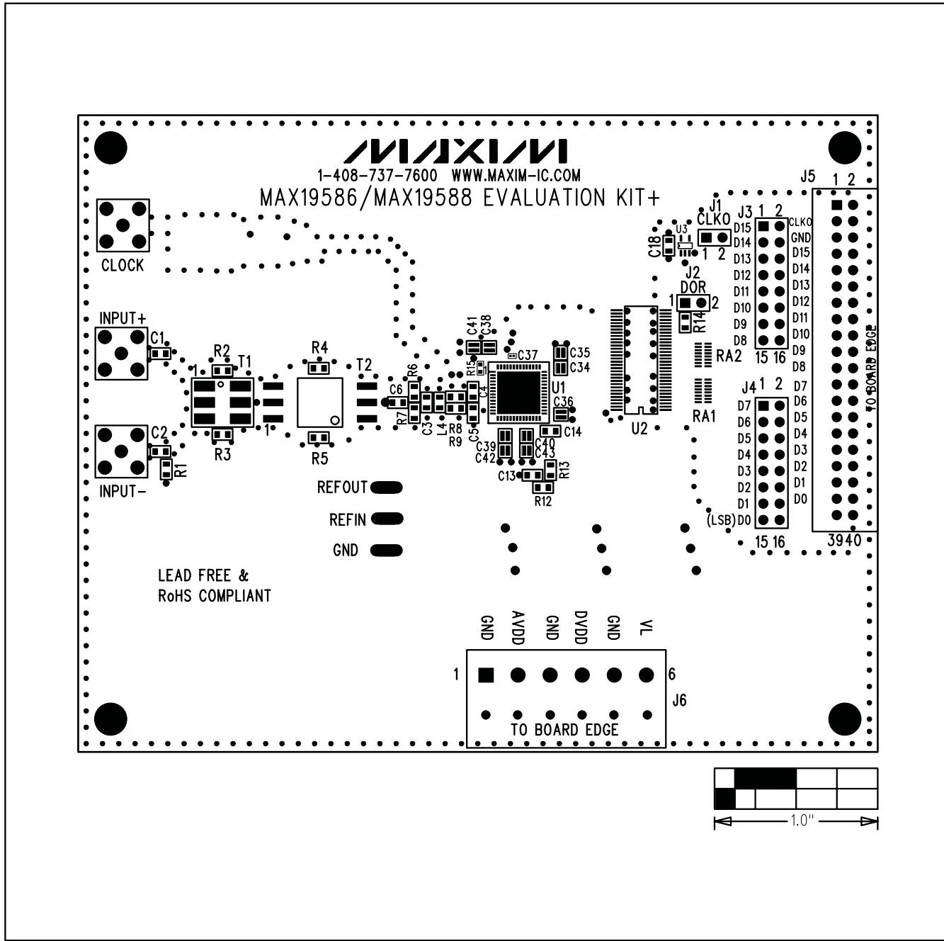
Figure 3. MAX19586/MAX19588 EV Kits Component Placement Guide—Component Side
