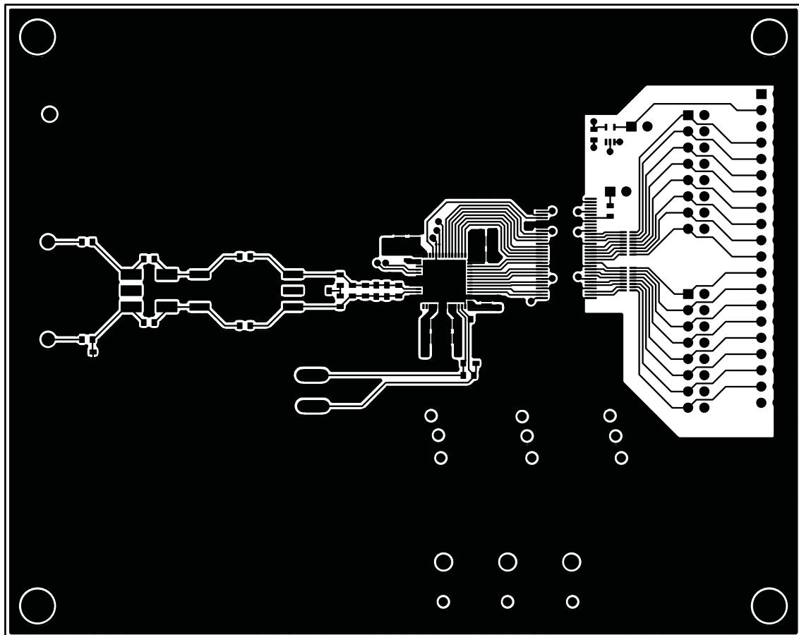
Figure 4. MAX19586/MAX19588 EV Kits PCB Layout—Component Side
