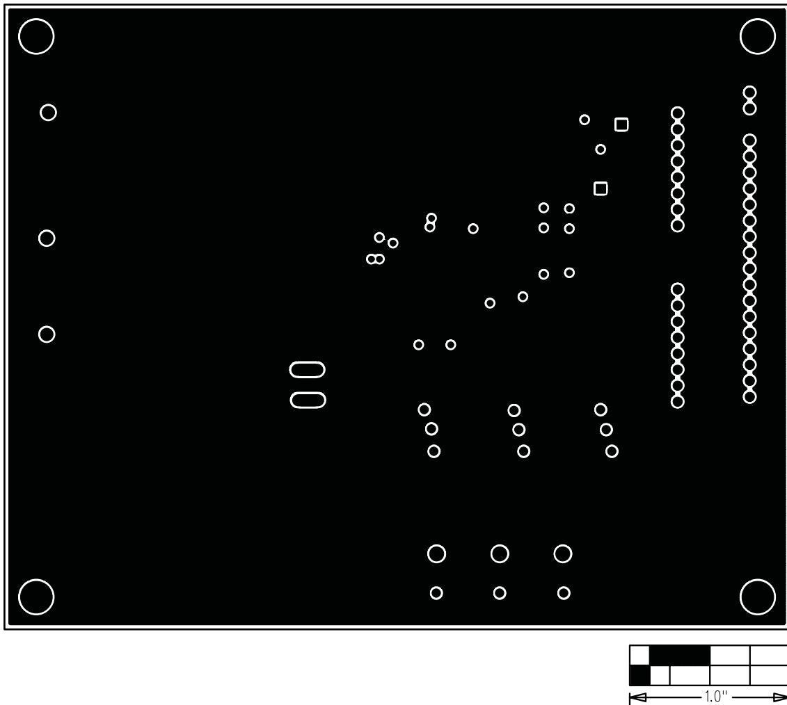
Figure 8. MAX19586/MAX19588 EV Kits PCB—GND Layer 5
