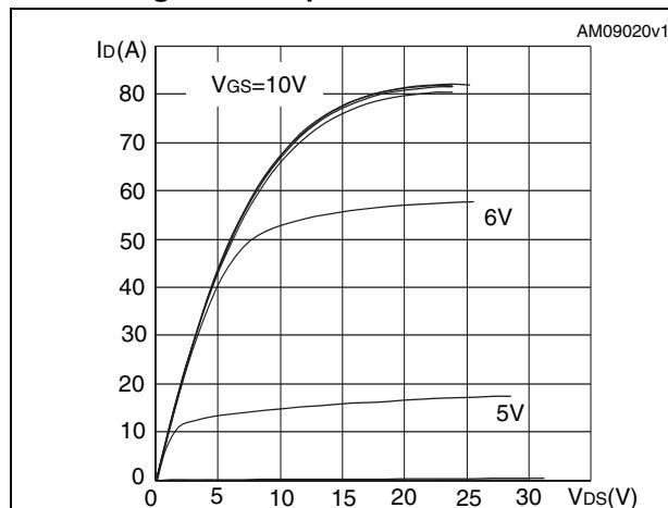
Figure 5. Transfer characteristics
