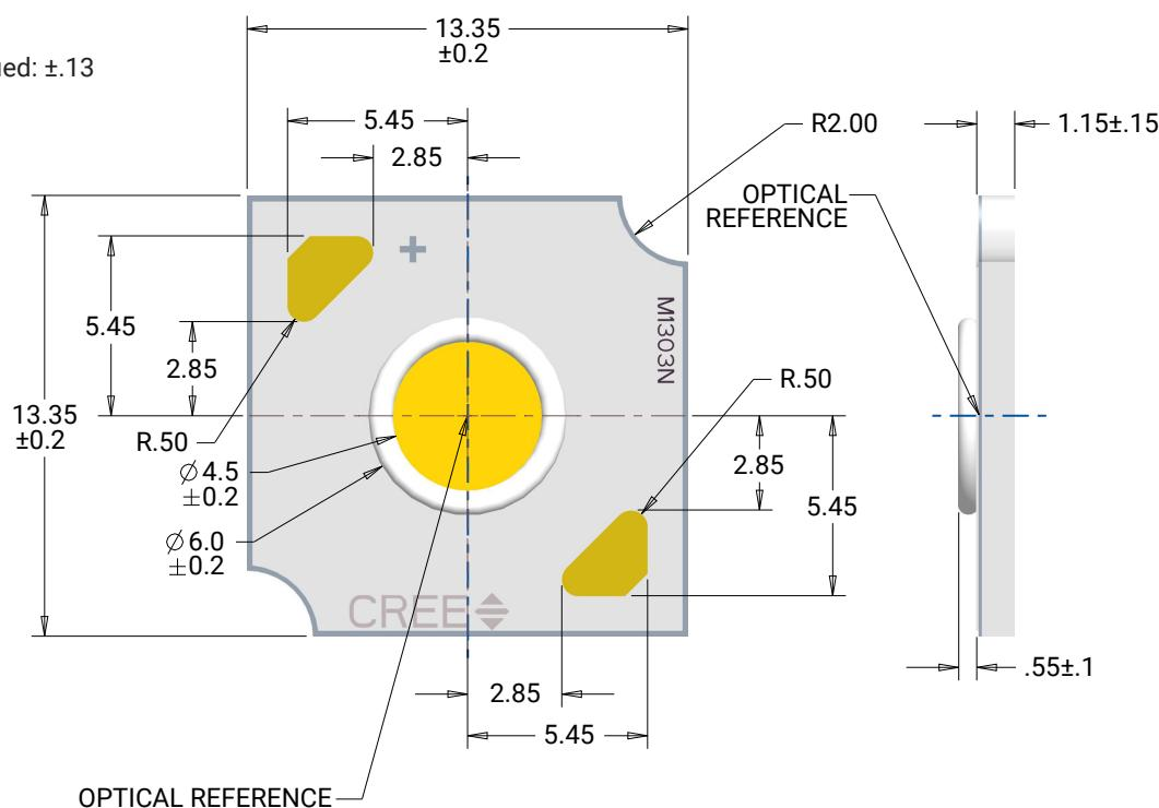
Tc measurement point: either the anode or cathode solder pad
