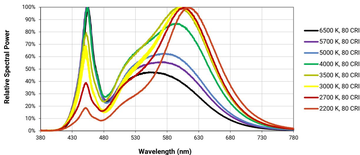
**RELATIVE SPECTRAL POWER DISTRIBUTION - STANDARD LEDs (CONTINUED)**
