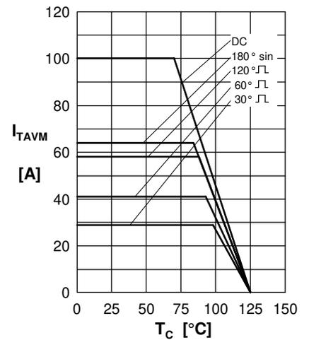
Fig. 3 Max. forward current at case temperature
