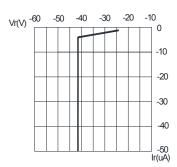
FIG.3 RED&AMBER REVERSE CURRENT VS. REVERSE VOLTAGE.
