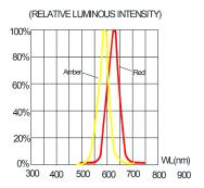
FIG.4 RELATIVE LUMINOUS INTENSITY VS. WAVELENGTH.
