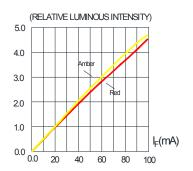
FIG.2 RELATIVE LUMINOUS INTENSITY VS. FORWARD CURRENT
