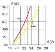
FIG.1 FORWARD CURRENT VS. FORWARD VOLTAGE.
