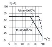
FIG.5 RED&AMBER MAXIMUM FORWARD DC CURRENT VS AMBIENT TEMPERATURE (Tjmax=110  $^{\circ}\mathrm{C})$
