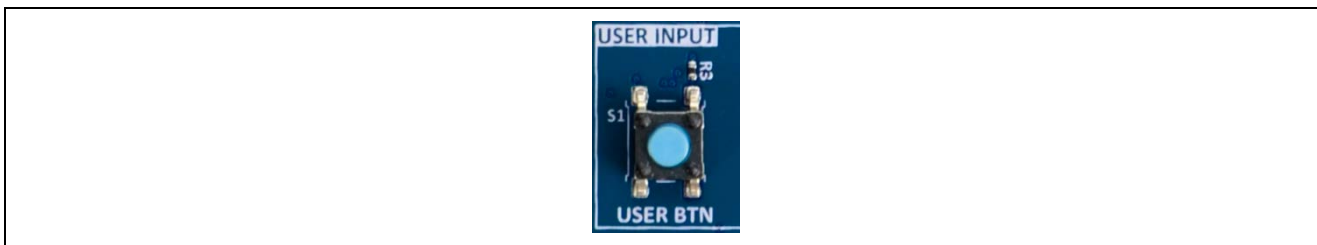
Figure 16. User Switch (S1) on Target Board
