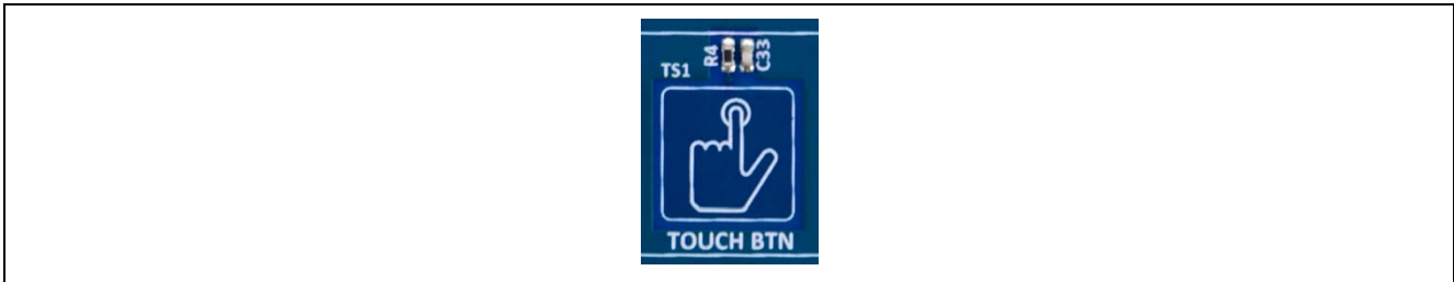
Figure 21. Capacitive Touch Button on Target Board (Top side)
