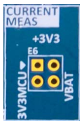
Figure 12. E6 on Target Board (Top Side)
