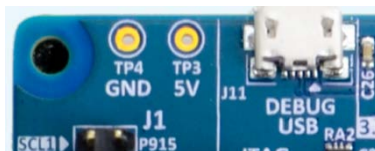
Figure 6. USB Debug Connector (J11), TP3, and TP4 on Target Board
