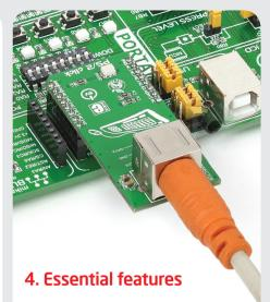
Even though somewhat superseded by USB, PS/2 connectors are still used. PS/2 click<sup>™</sup> is especially suited for connecting vintage or certain modern high-end keyboards and mice. One of the key benefits of PS/2 is that it supports full n-key rollover. It's the ability of the keyboard to handle any number of simultaneous keystrokes.
