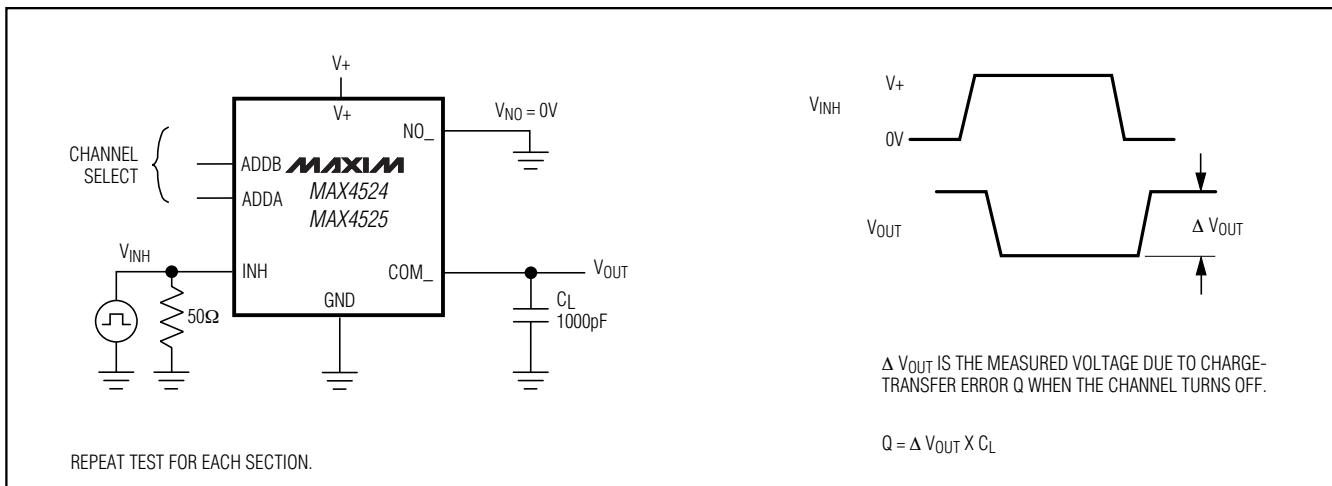
Figure 4. Charge Injection
