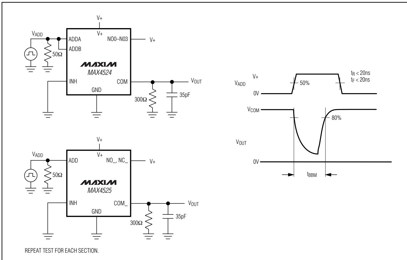
Figure 3. Break-Before-Make Interval
