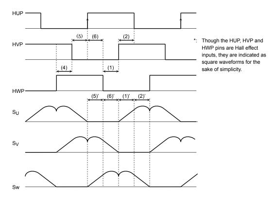
As illustrated above, the modulated waveform ) (1)'advances by 1/32 of the period between the rising edge ( $\checkmark$ ) of HU and the falling edge ( $\checkmark$ ) of HW. Likewise, the modulated waveform (2)' advances by 1/32 of the period between the falling edge ( $\checkmark$ ) of HW and the rising edge ( $\checkmark$ ) of HV.
