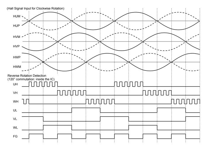
\*: If the Hall signal for clockwise rotation is applied when CW/CCW = High, the motor is driven by the 120° commutation signal with a lead angle of 0°. (Reverse rotation by the wind)
