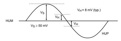
\*: The Hall amplifier can operate when V<sub>S</sub> is at least 50mVpp. However, to stabilize the time interval between zero-cross points of each phase signal, that is, the 60-electrical-degree interval, the amplitude should be as high as possible. (VS is recommended to be 200 mVpp or higher.)
