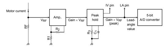
\*: Gain = (R<sub>1</sub> + R<sub>2</sub>) /R<sub>1</sub>, R<sub>3</sub> = 100 kΩ, C<sub>1</sub> = 0.1  $\mu$ F
