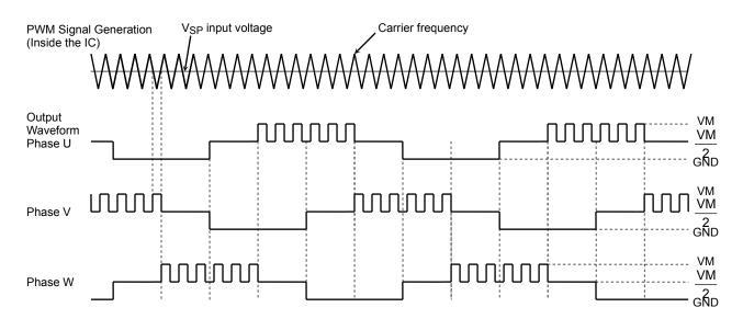
Note: The above U-phase waveform shows the behavior of the U-phase output signal when a resistor is connected between the U and VM pins and also between the U pin and ground to obtain  $\frac{VM}{2}$ . Likewise, resistors are connected to the V and W pins.  $\frac{VM}{2}$  indicates the high-impedance state.
