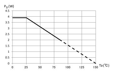
Measured on a board (100 mm  $\times$  100 mm  $\times$  t1.5 mm, Double-layers) Rth (j-a) = 32°C/W
