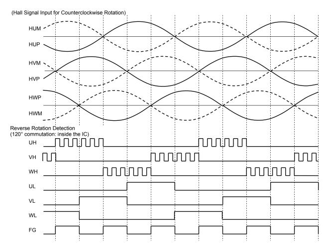
\*: If the Hall signal for counterclockwise rotation is applied when CW/CCW = Low, the motor is driven by the 120° commutation signal with a lead angle of 0°. (Reverse rotation by the wind)
