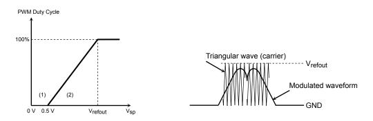
Note: An amplitude of the modulated waveform becomes maximum when V<sub>SP</sub> = V<sub>refout</sub>. The PWM duty cycle that is obtained with the V<sub>SP</sub> voltage of V<sub>refout</sub> is defined as 100%.
