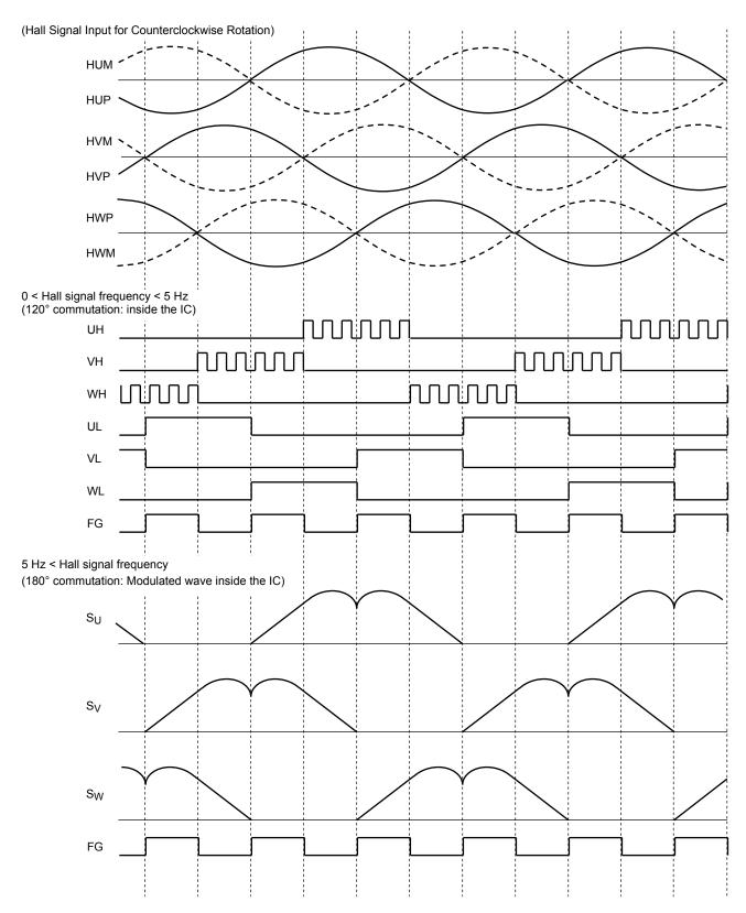
\*: The lead-angle correction is performed in accordance with the LA input when the Hall signal frequency is 2.5 Hz or higher.
