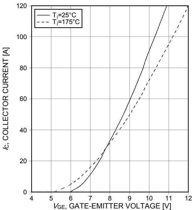
**Figure 7. Typical transfer characteristic**
