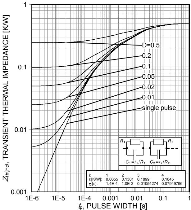
**Figure 19.** IGBT transient thermal impedance
