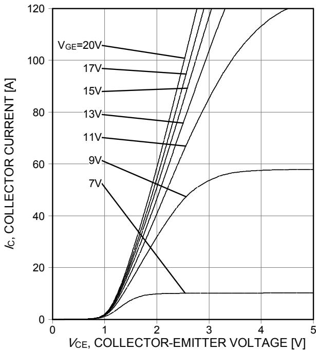
**Figure 5. Typical output characteristic**
