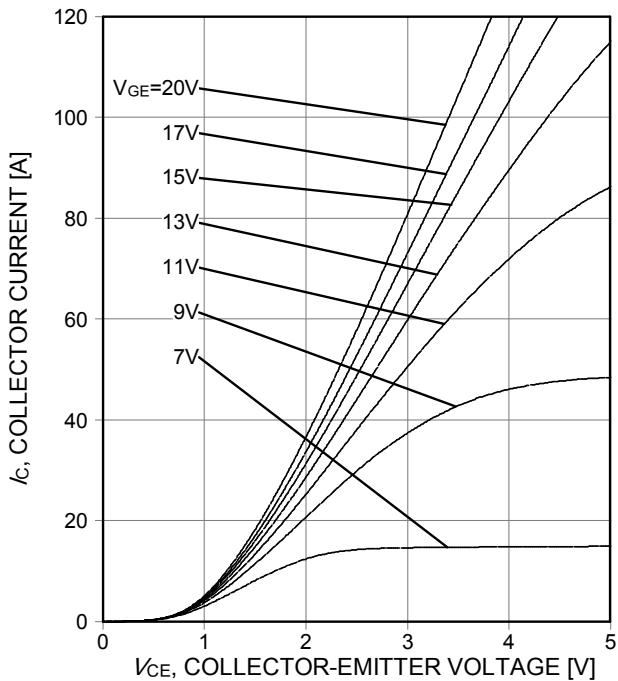
**Figure 6. Typical output characteristic**
