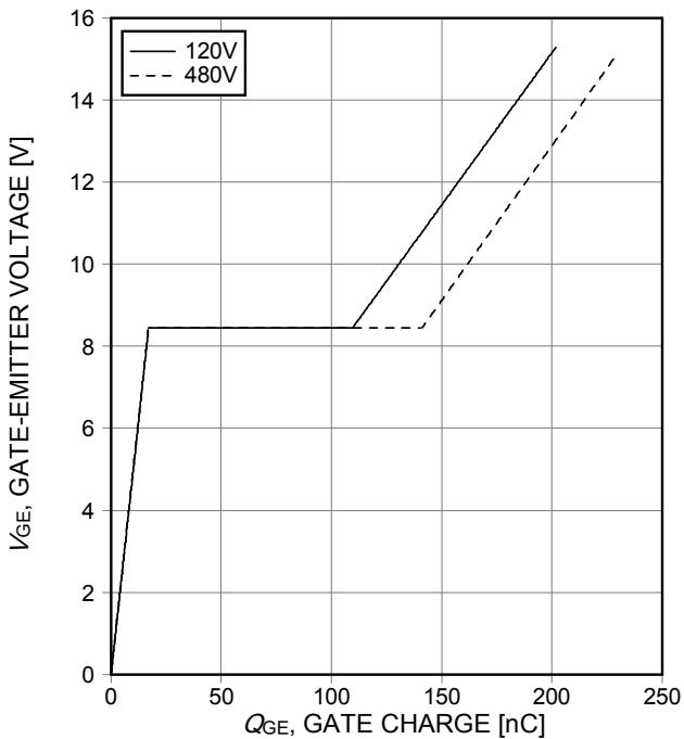
**Figure 17.** Typical gate charge
