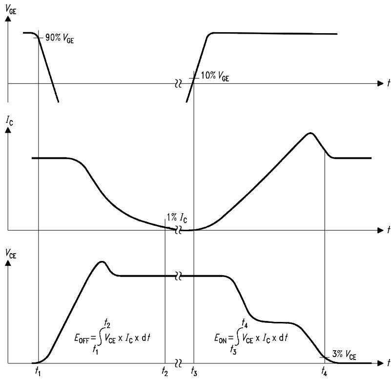
**Figure B. Definition of switching losses**
