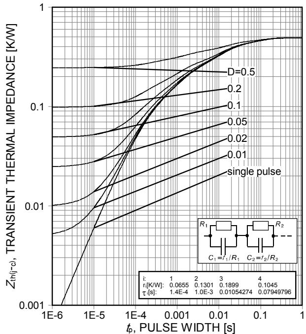
**Figure 20.** Diode transient thermal impedance as a function of pulse width
