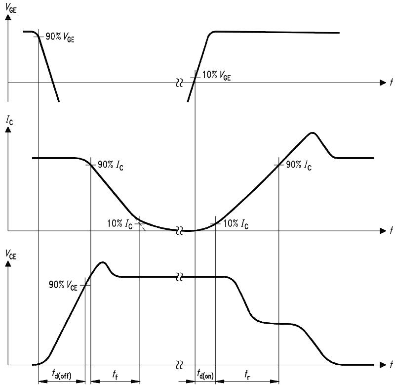
**Figure A. Definition of switching times**
