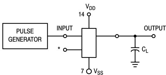
\*All unused inputs of AND, NAND gates must be connected to V<sub>DD</sub>.
