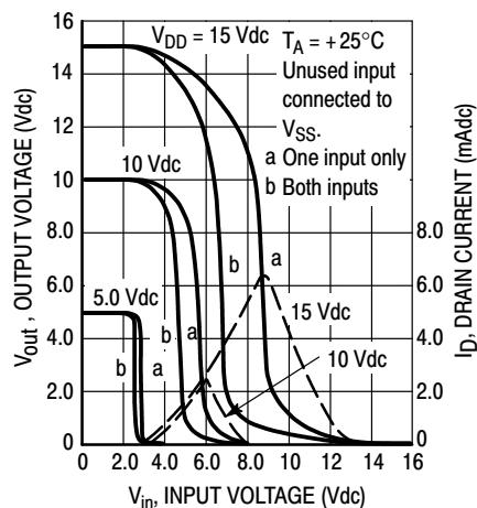
**Figure 2. Typical Voltage and Current Transfer Characteristics**
