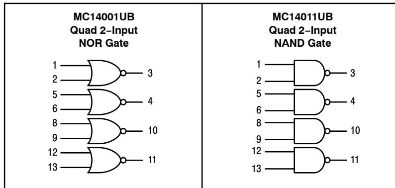
$V_{DD}$  = PIN 14
