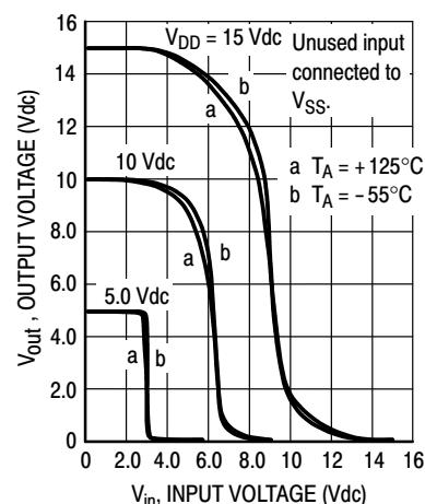
**Figure 3. Typical Voltage Transfer Characteristics versus Temperature**
