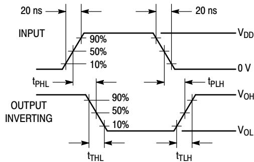
Figure 1. Switching Time Test Circuit and Waveforms
