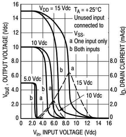
**Figure 2. Typical Voltage and Current Transfer Characteristics**
