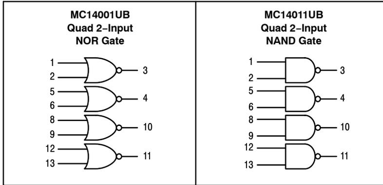
$V_{DD}$  = PIN 14
