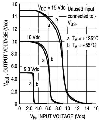
**Figure 3. Typical Voltage Transfer Characteristics versus Temperature**
