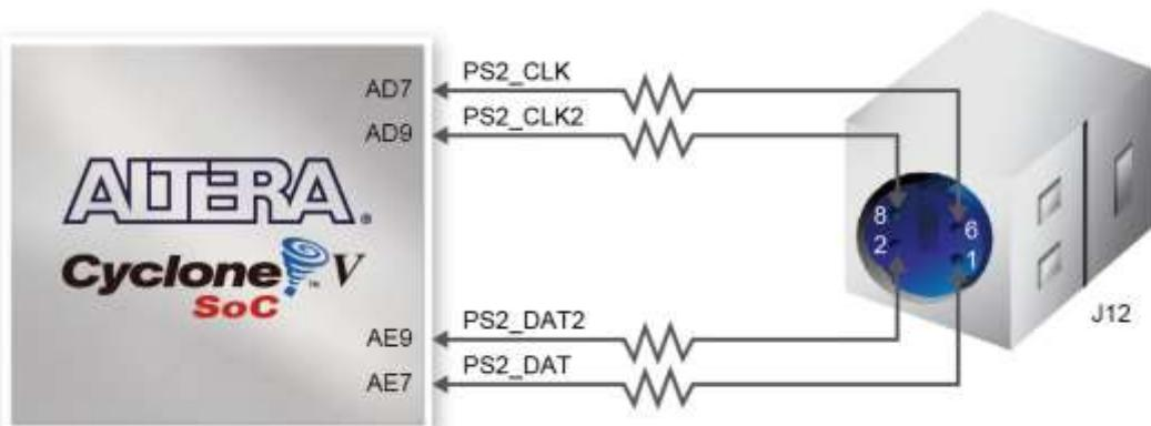
**Figure 3-29 Connections between the FPGA and PS/2**
