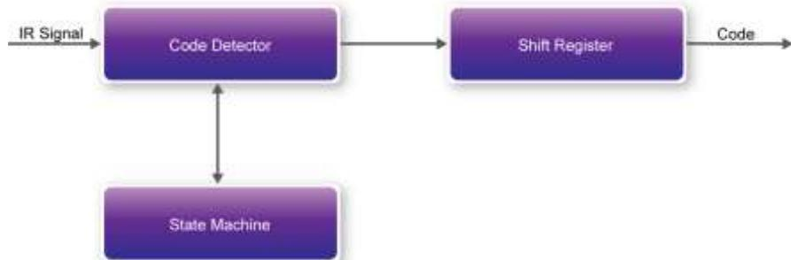
**Figure 5-19 Modules in the IR Receiver controller**
