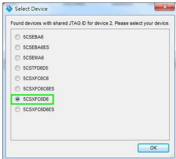
**Figure 3-4 Select 5CSXFC6D6 device**
