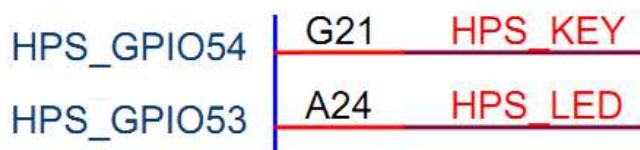
**Figure 6-4 Pin assignment of LED and KEY**
