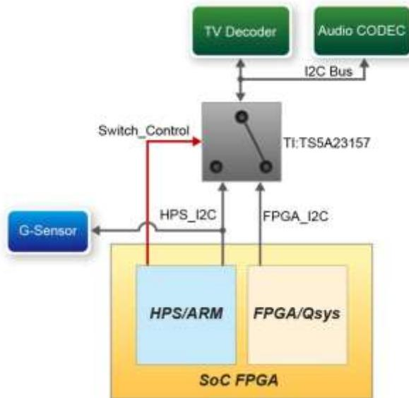
**Figure 3-22 Control mechanism for the I2C multiplexer**
