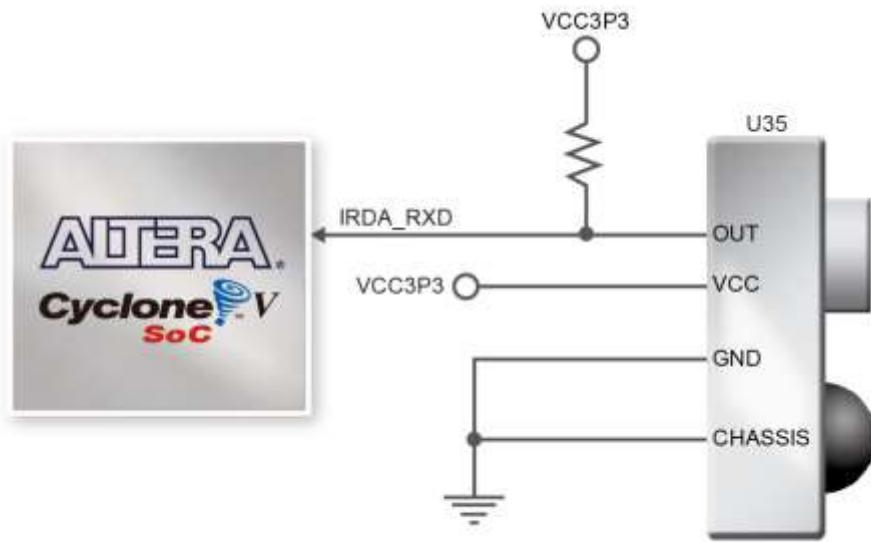
Figure 3-26 Connection between the FPGA and IR Receiver
