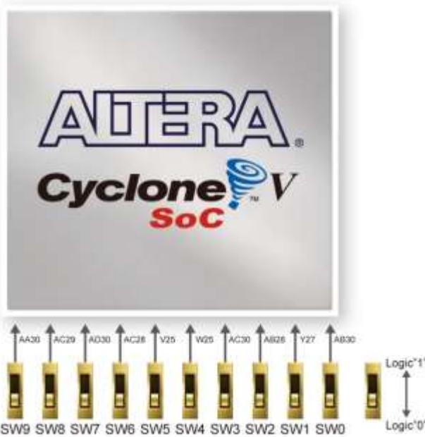
**Figure 3-16 Connections between the slide switches and the Cyclone V SoC FPGA**
