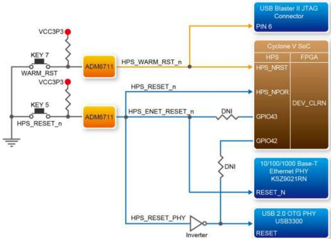
**Figure 3-12 HPS reset tree on DE10-Standard board**
