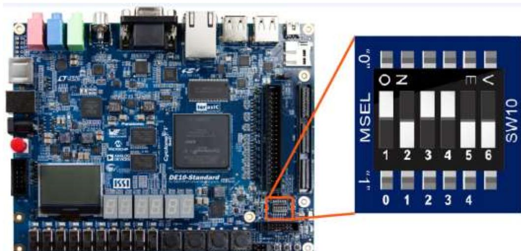
Figure 3-1 DIP switch (SW10) setting of Active Serial (AS) mode on DE10-Standard board
