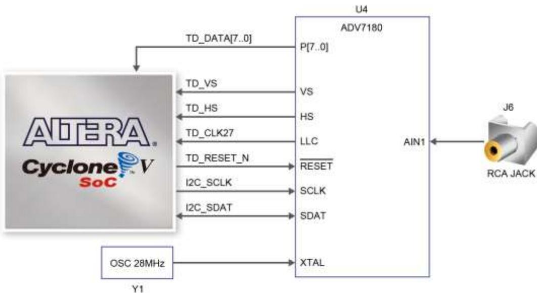
**Figure 3-25 Connections between the FPGA and TV Decoder**
