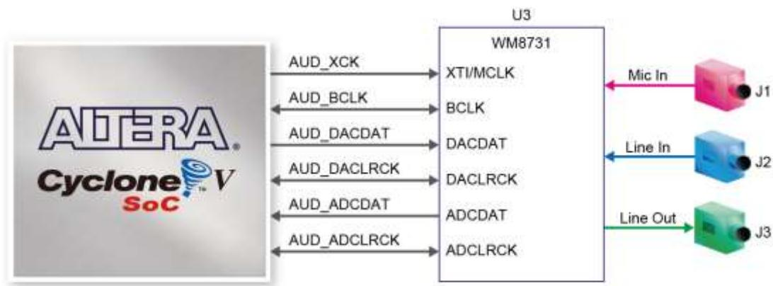
Figure 3-21 Connections between the FPGA and audio CODEC
