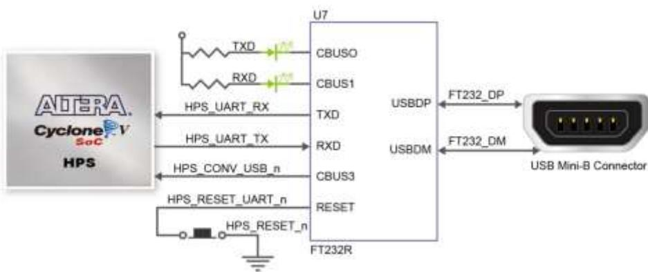
**Figure 3-34 Connections between the HPS and FT232R Chip**
