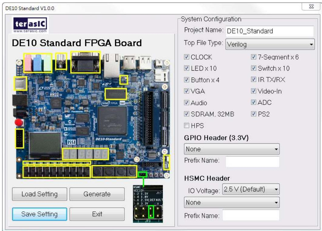
**Figure 4-2 The GUI of DE10-Standard System Builder**
