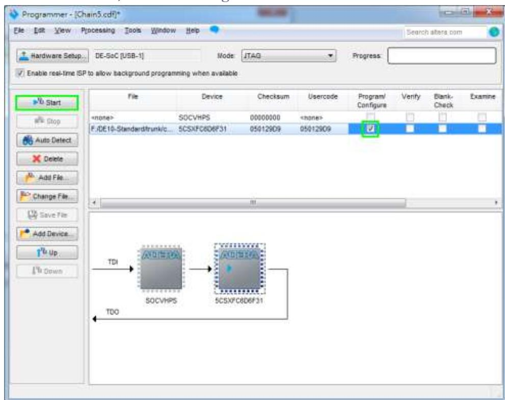
**Figure 3-8 Program .sof file into the FPGA device**
