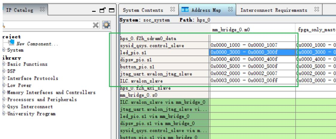
**Figure 7-2** FPGA peripherals address map
