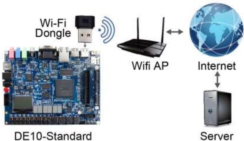
Figure 6-15 System diagram of USB Wi-Fi dongle
