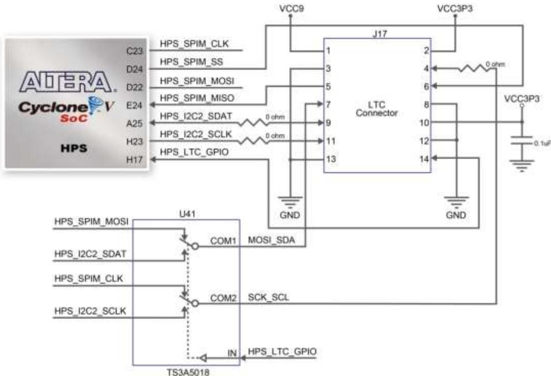
**Figure 3-39 Connections between the HPS and LTC connector**
