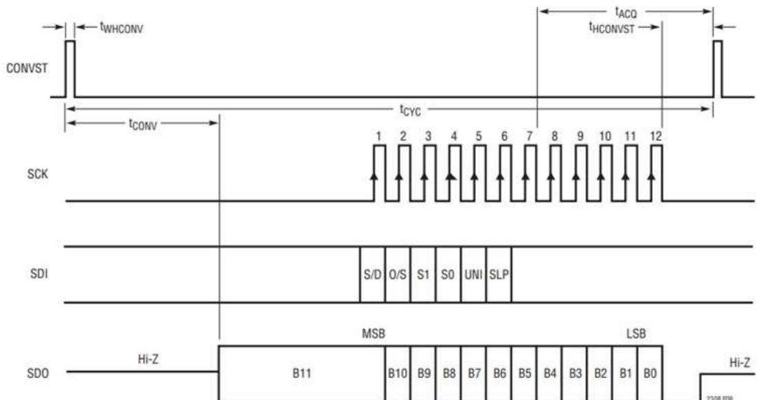
**Figure 5-23 LTC2308 Timing with a Short CONVST Pulse**
