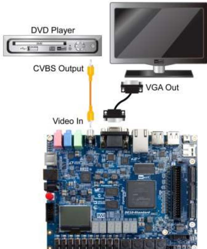
**Figure 5-12 Setup for the TV box demonstration (VIP)**
