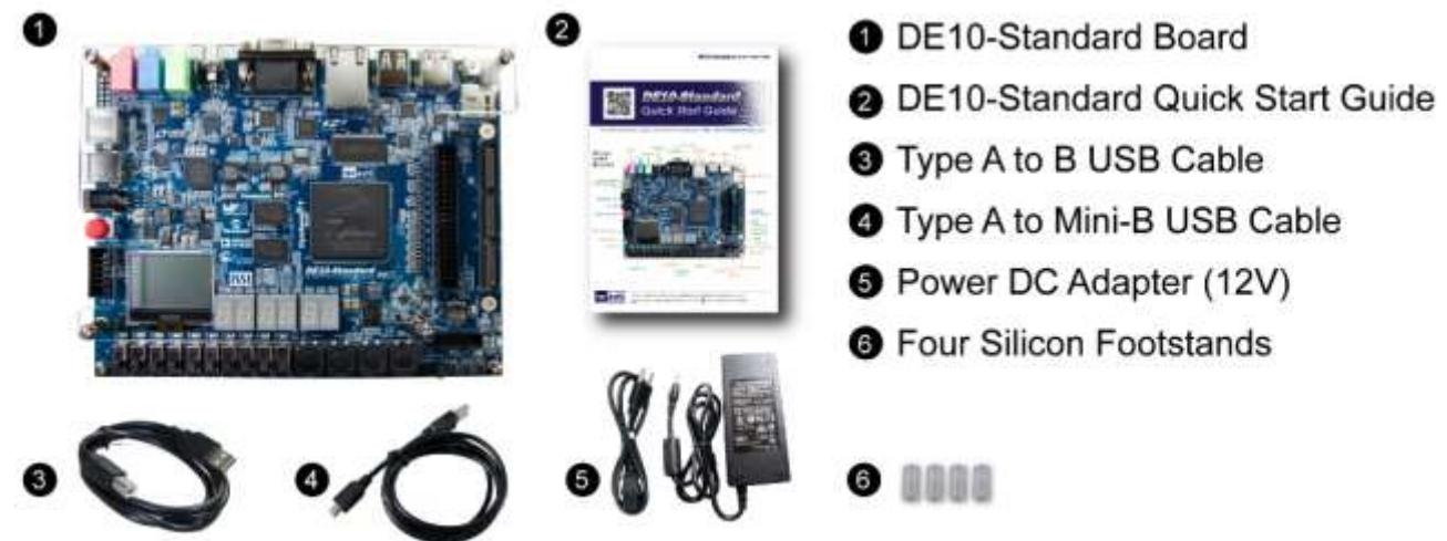
Figure 1-1 The DE10-Standard package contents
