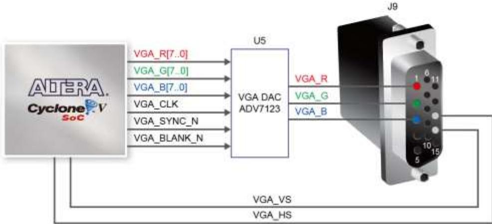
**Figure 3-23 Connections between the FPGA and VGA**
