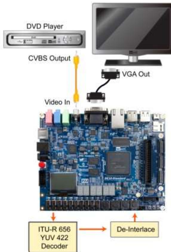
**Figure 5-10 Setup for the TV box demonstration**
