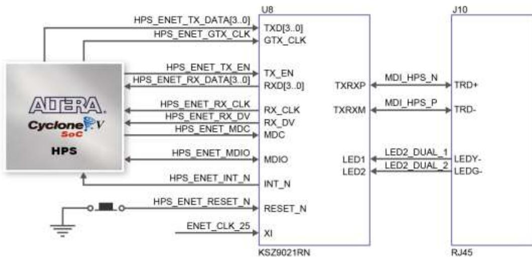
**Figure 3-33** Connections between the HPS and Gigabit Ethernet
