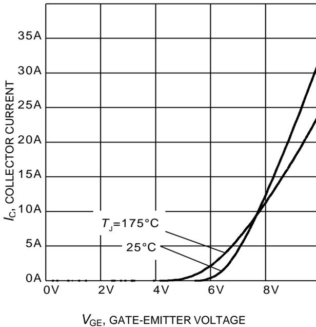
**Figure 7. Typical transfer characteristic**
