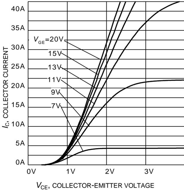
**Figure 5. Typical output characteristic**
