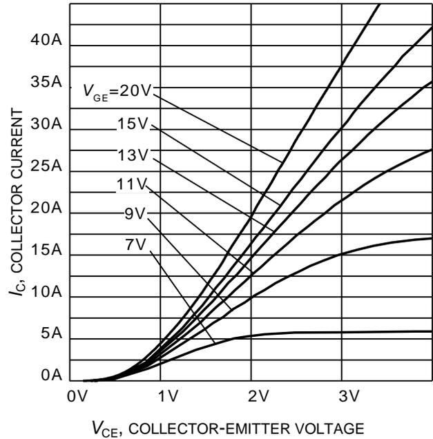
**Figure 6. Typical output characteristic**
