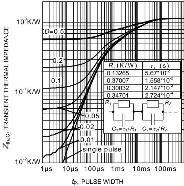
**Figure 21. IGBT transient thermal impedance**
