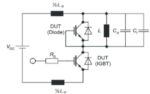
**Figure E. Dynamic test circuit**
