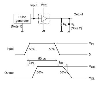
Note 1: Pulse width 50  $\mu$ s, Duty cycle 10% Output impedance 50  $\Omega$ , t<sub>r</sub> ≤ 5 ns, t<sub>f</sub> ≤ 10 ns, V<sub>IH</sub> = 5.0 V
