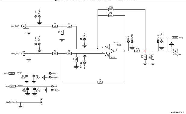
Figure 1. STEVAL-CCA036V1 internal circuit
