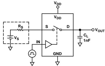
Figure 24. Charge Injection
