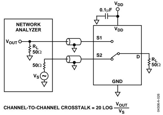
Figure 27. Channel-to-Channel Crosstalk
