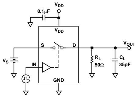
Figure 23. Switching Times
