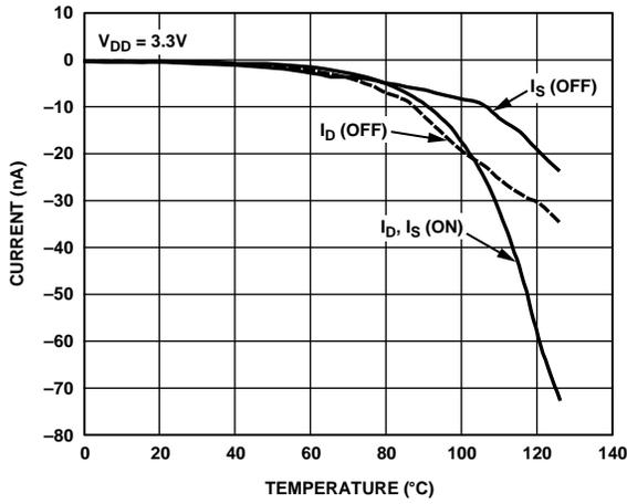
Figure 11. Leakage Current vs. Temperature,  $V_{DD} = 3.3V$
