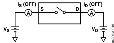
Figure 21. Off Leakage
