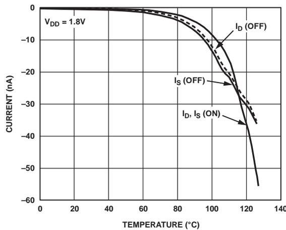
Figure 13. Leakage Current vs. Temperature,  $V_{DD} = 1.8V$
