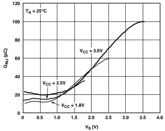
Figure 14. Charge Injection ( $Q_{INJ}$ ) vs. Source Voltage ( $V_S$ )
