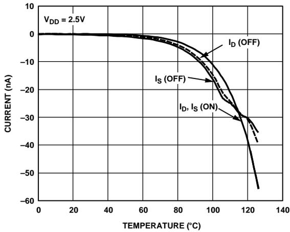
Figure 12. Leakage Current vs. Temperature,  $V_{DD} = 2.5V$
