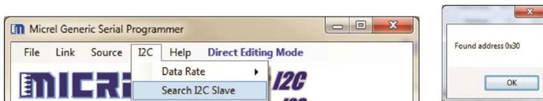
Figure 13. Searching for an I<sup>2</sup>C Slave Device
