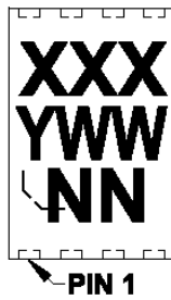
14-Lead SOIC (150 mil) (MCP6H94)
