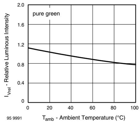
Figure 25. Rel. Luminous Intensity vs. Ambient Temperature
