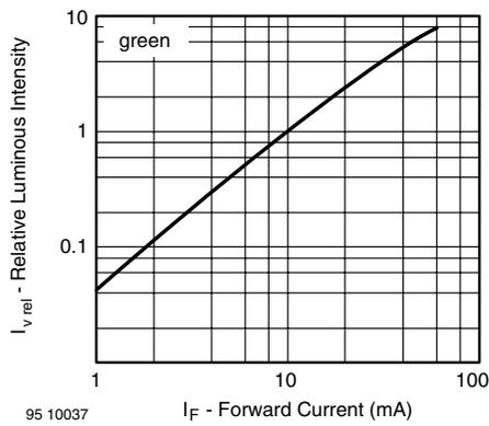
Figure 22. Relative Luminous Intensity vs. Forward Current
