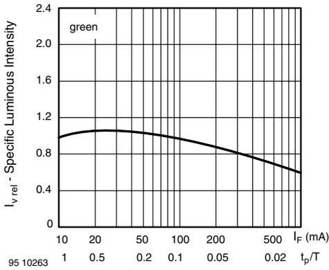
Figure 21. Specific Luminous Intensity vs. Forward Current
