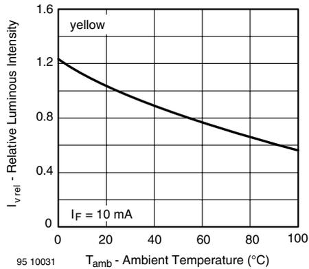
Figure 15. Rel. Luminous Intensity vs. Ambient Temperature
