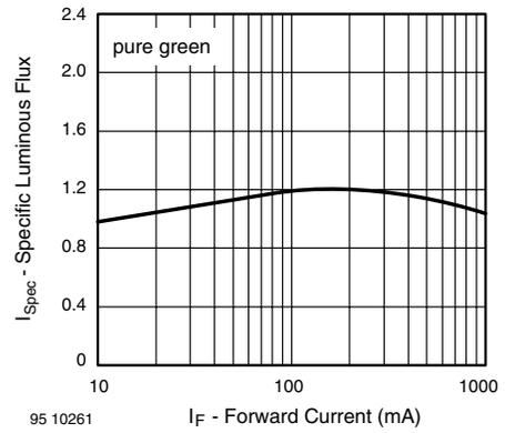
Figure 26. Specific Luminous Intensity vs. Forward Current
