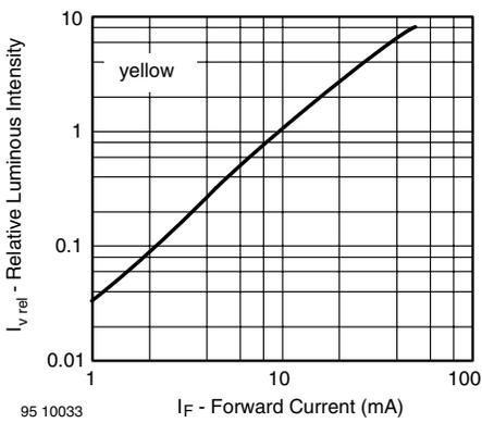
Figure 17. Relative Luminous Intensity vs. Forward Current
