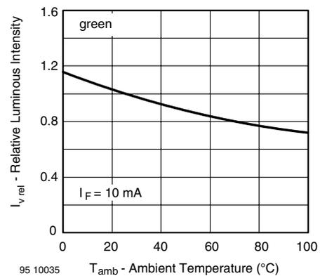
Figure 20. Rel. Luminous Intensity vs. Ambient Temperature
