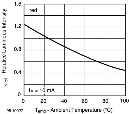
Figure 10. Rel. Luminous Intensity vs. Ambient Temperature
