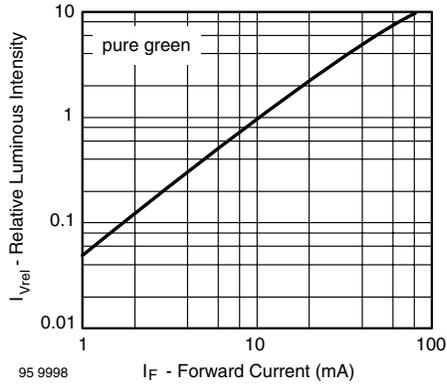
Figure 27. Relative Luminous Intensity vs. Forward Current
