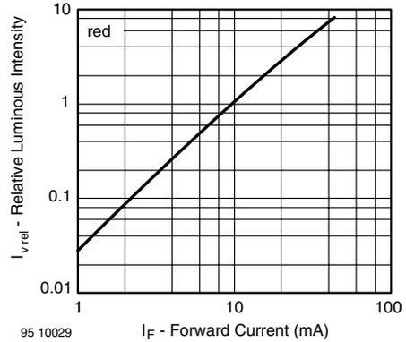
Figure 12. Relative Luminous Intensity vs. Forward Current
