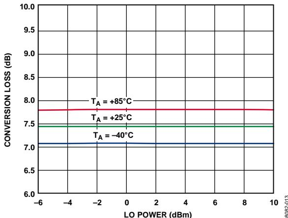
Figure 18. Power Conversion Loss vs. LO Power
