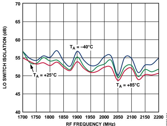
Figure 29. LO Switch Isolation vs. RF Frequency
