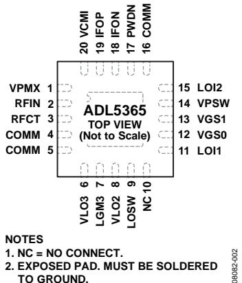
Figure 2. Pin Configuration
