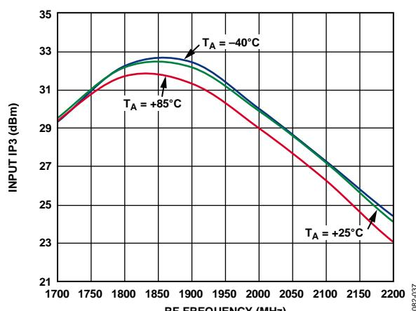
Figure 40. Input IP3 vs. RF Frequency at 3.3 V
