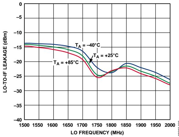
Figure 31. LO to IF Leakage vs. LO Frequency
