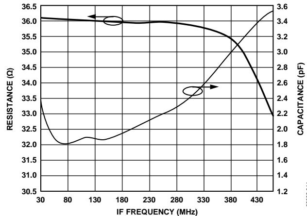
Figure 26. IF Output Impedance ( $R$  Parallel,  $C$  Equivalent)
