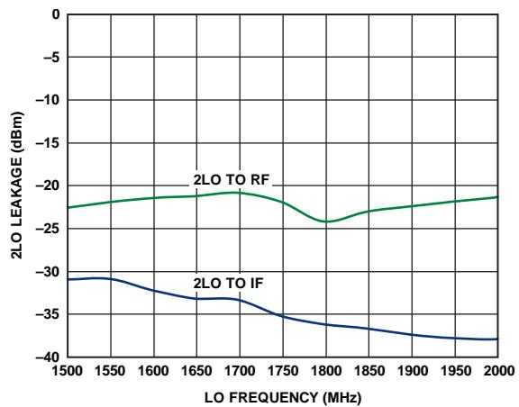
Figure 33. 2LO Leakage vs. LO Frequency
