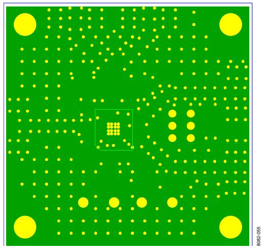
Figure 51. Evaluation Board Ground Plane, Internal Layer 1
