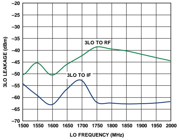
Figure 34. 3LO Leakage vs. LO Frequency
