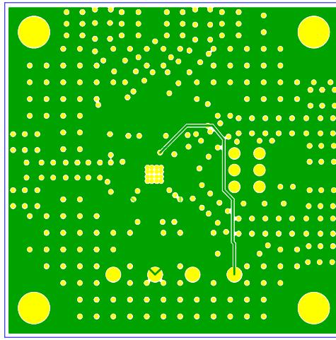
Figure 52. Evaluation Board Power Plane, Internal Layer 2
