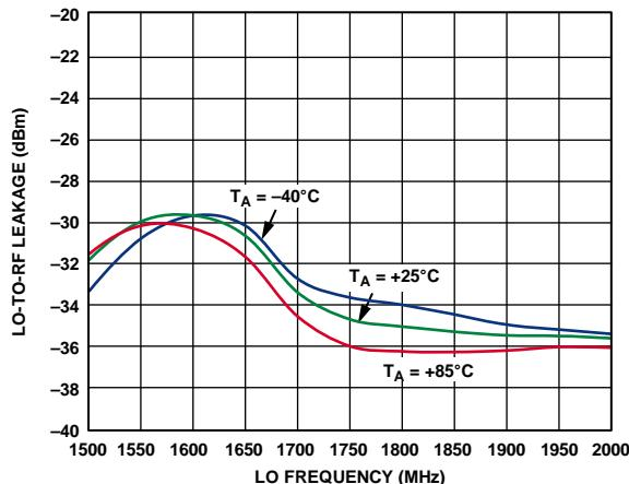
Figure 32. LO to RF Leakage vs. LO Frequency
