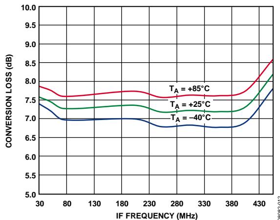
Figure 14. Power Conversion Loss vs. IF Frequency
