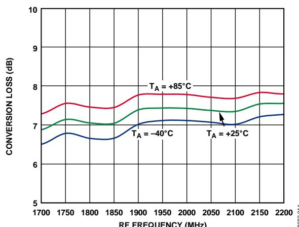
Figure 4. Power Conversion Loss vs. RF Frequency
