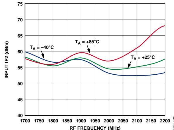
Figure 41. Input IP2 vs. RF Frequency at 3.3 V
