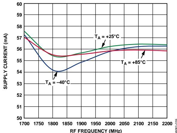
Figure 38. Supply Current vs. RF Frequency at 3.3 V
