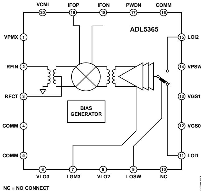
Figure 47. Simplified Schematic
