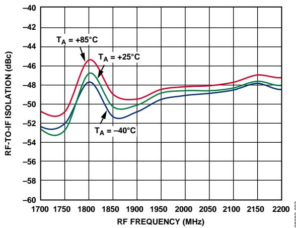
Figure 30. RF to IF Isolation vs. RF Frequency
