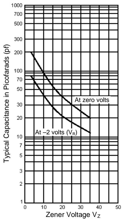
**FIGURE 3** – Capacitance vs. Zener Voltage (Typical)
