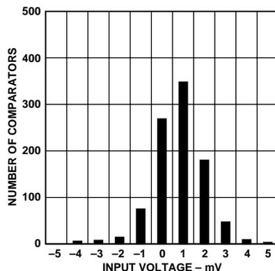
Figure 2. Typical Distribution of Input Offset Voltage
