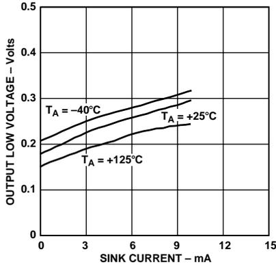
Figure 10. Output Low Voltage,  $V_{OL}$  vs. Sink Current
