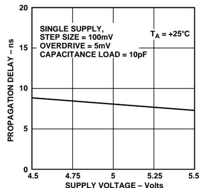
Figure 6. Propagation Delay vs. Positive Supply Voltage
