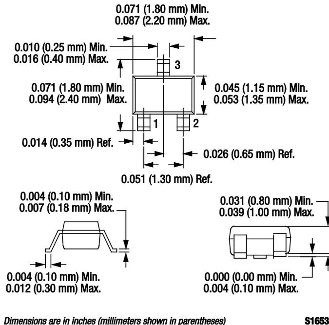
Figure 10. SC-70 Package Dimension Drawing
