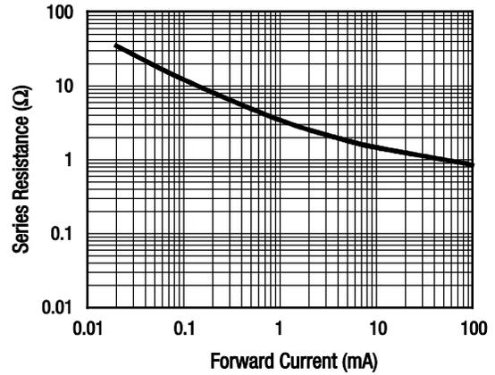
Figure 2. Series Resistance vs Current @ 100 MHz
