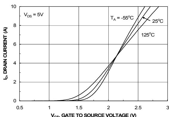
**Figure 5. Transfer Characteristics**
