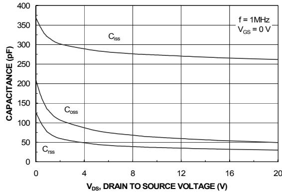
**Figure 8. Capacitance Characteristics**
