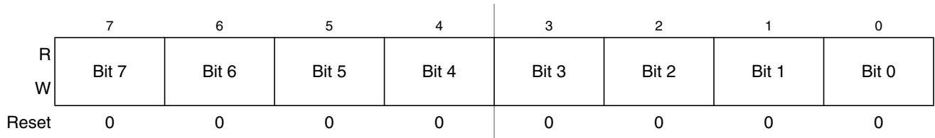
Figure 7-18. Debug Comparator A Register Low (DBGCAL)
