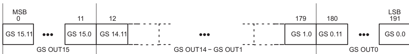
Figure 17. Grayscale Data Packet Format
