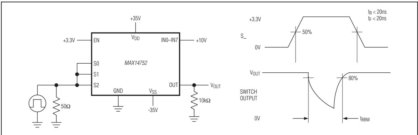
Figure 6. Break-Before-Make Interval
