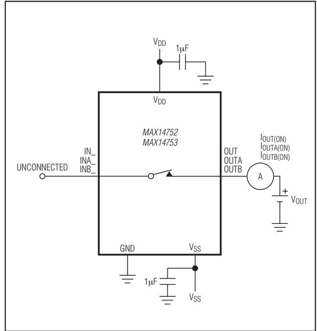
Figure 2. On-Leakage Current
