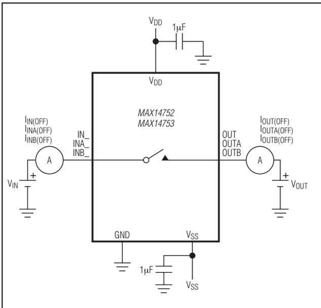
Figure 3. Off-Leakage Current
