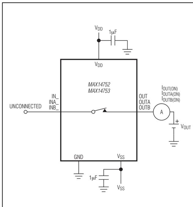
Figure 2. On-Leakage Current
