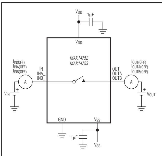
Figure 3. Off-Leakage Current
