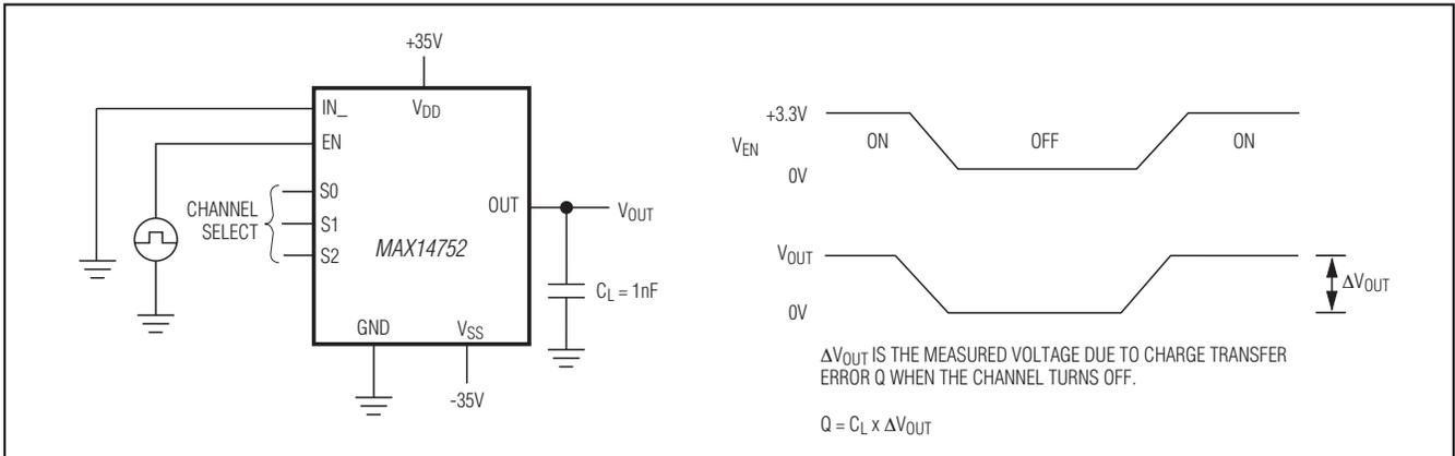
Figure 10. Charge Injection
