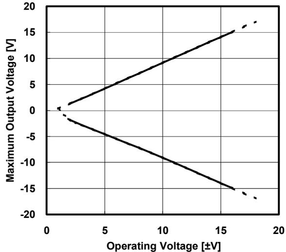
**Maximum Output Voltage vs. Operating Current**
