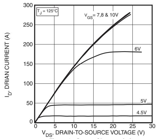
Figure 2, Output Characteristics
