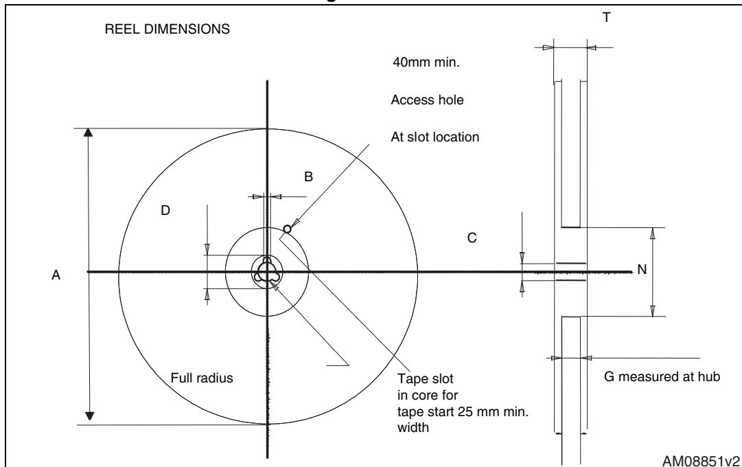
Table 9. D<sup>2</sup>PAK (TO-263) tape and reel mechanical data
