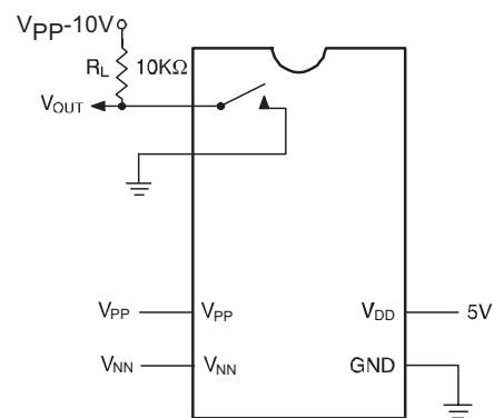
$T_{ON}/T_{OFF}$  Test Circuit
