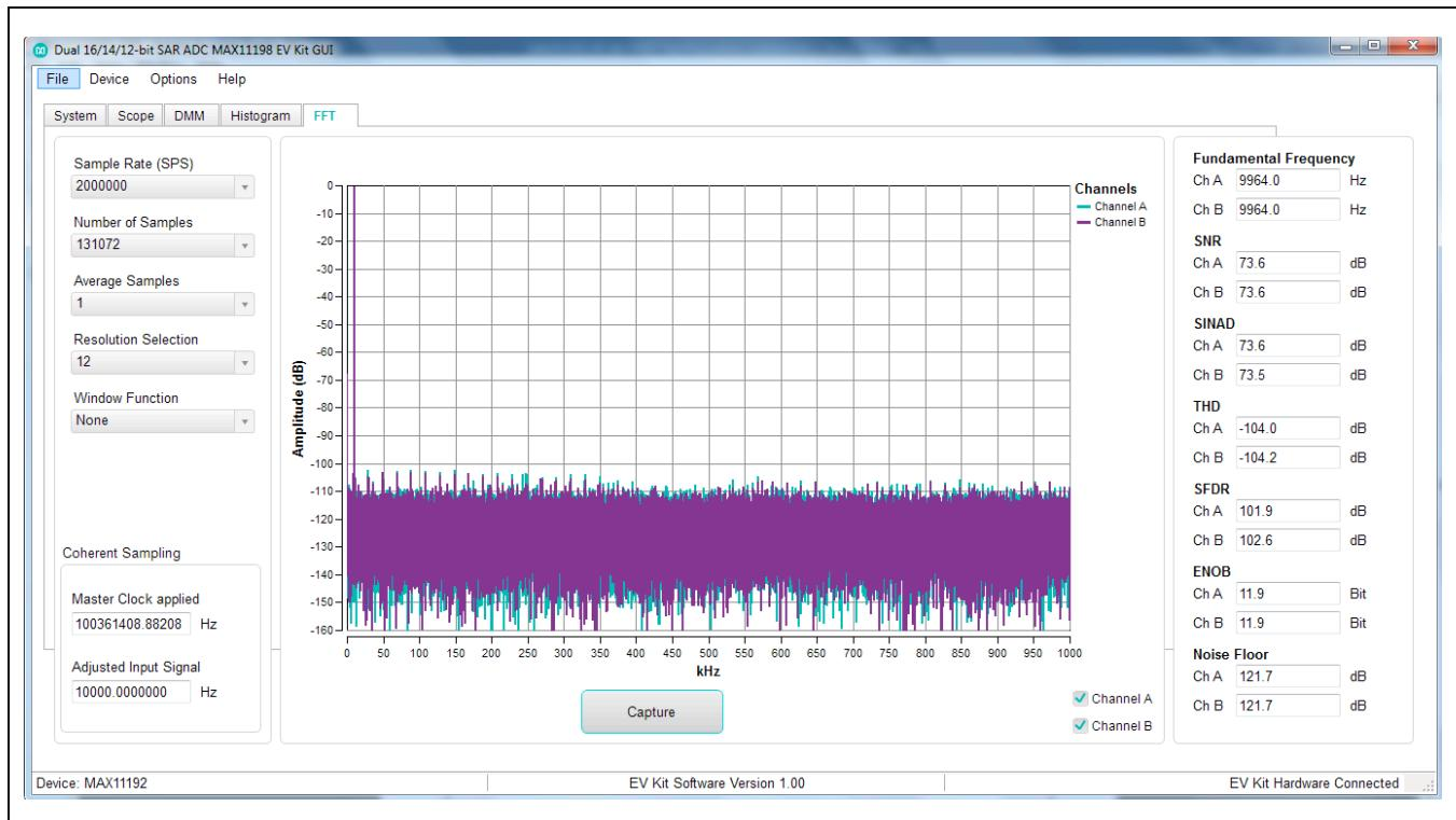
Figure 7. MAX11192 EV Kit Coherent Sampling (FFT Tab)
