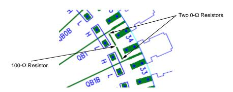
Figure 2. LVDS Output Configuration
