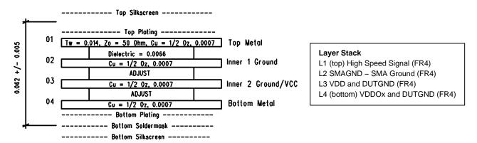
Figure 10. QFN-48 Evaluation Board Layout, 4-Layer Stack
