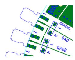
Figure 4. LVPECL Output Configuration
