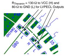
Figure 5. LVPECL Output Configuration, Thevenin Termination Resistors
