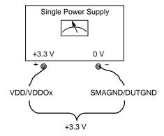
Figure 8. Single Power Supply Configuration
