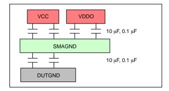
Figure 11. Typical Power Supply By-Pass
