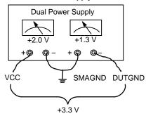
Figure 6. LVPECL – "Split" or Dual Power Supply Configuration
