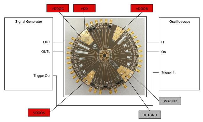
Figure 9. Typical Lab Test Set-Up
