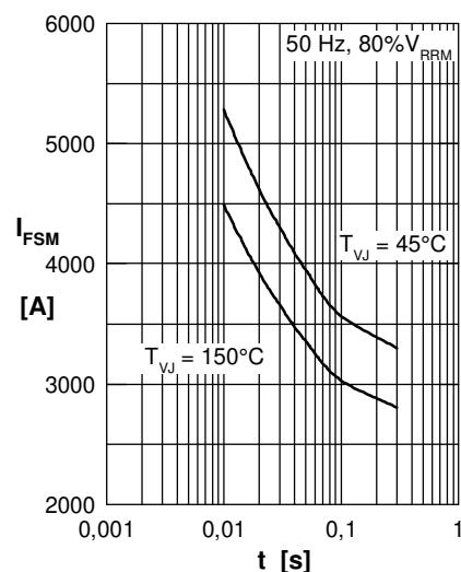
Fig. 2 Surge overload current vs. time per diode
