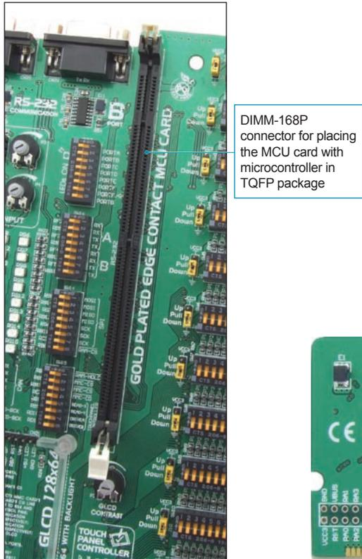
Figure 2-1: DIMM-168P connector
