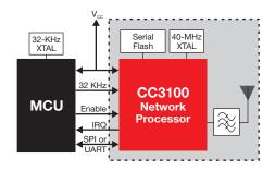
The CC3100 device is a Wi-Fi, self-contained network processor with on-chip web server and embedded TCP/IP stack that connects easily to any low-cost and low-power microcontroller (MCU) such as the MSP430F552, thanks to a simple UART or SPI driver and host memory footprint as low as 7kB of code to reside on the MCU. Hardware design is made easy for space-constrained boards with a small 64-pin 9×9 mm QFN package. Certified modules will
