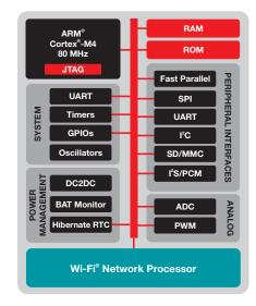
integrates a high-performance 80-MHz ARM® Cortex®-M4 MCU and peripherals allowing customers to develop their application with a single device. Developers can fully access the MCU portion with 200kB of application code available fully independent from the Wi-Fi processing. The peripheral set includes parallel camera, I²S audio, SDMMC, ADC, SPI, UART, I²C, PWM, I/Os, built-in power management and RTC enabling many MCU embedded applications to connect to the cloud.
