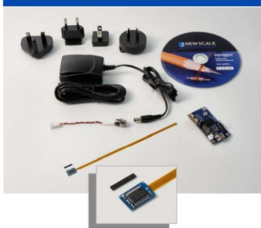
The TRK-1T02-E Evaluation Pack is a full-featured development platform for the NSE5310 Position Sensor. The MC-33MB interface card accepts the I<sup>2</sup>C input from one or two NSE5310 sensors, and connects via USB to your PC. Use the New Scale Pathway™ Software to view and collect position information. This development kit provides for easy sensor evaluation and system development.
